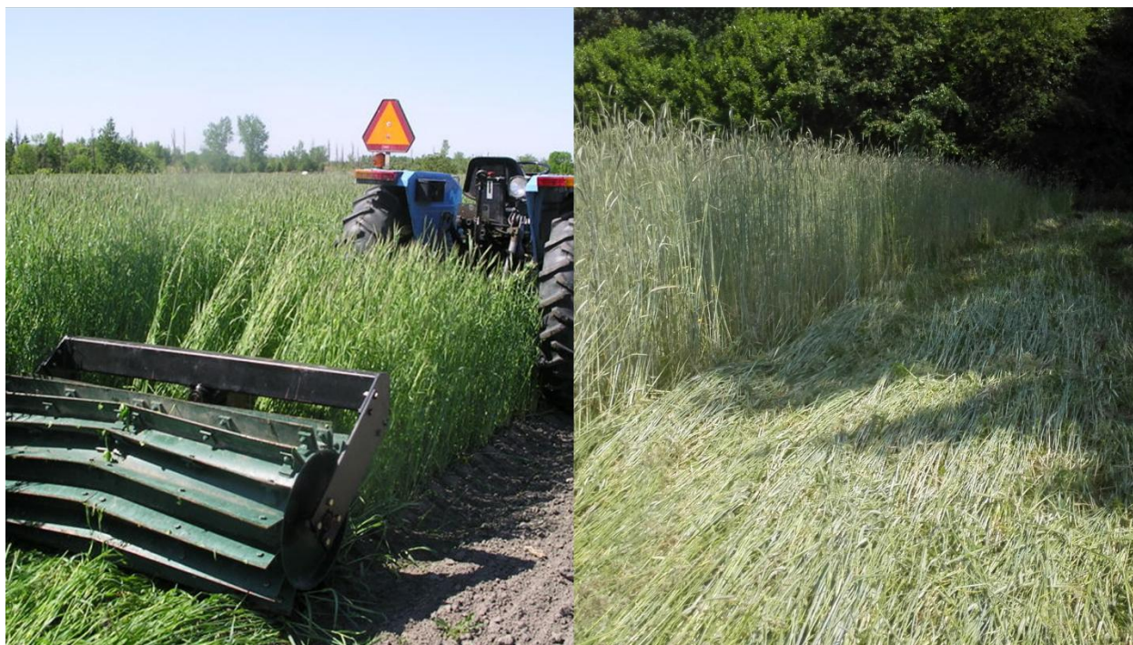
Fig. 6 Roller crimper (on the left) and vegetation lodged after the passage of the equipment (on the right side).
